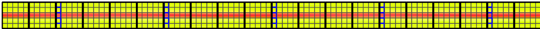
Fig. 3.3: This is how the focal plane instrumented with the scintillating fibers looks to the incoming electrons. The red stripe shows the beam intensity profile once it is centered on a row of fibers. Light gray lines show the segmentation of individual fibers, thick black lines indicate boundaries between fiber bundles. In this segmentation plan a bundle has 25 fibers, which can be read-out by a single 30-channel SiPM amplifier board. Note that other segmentation plans are possible; in all cases, the electronics allows for individual fiber readout in the edge column of any bundle.
