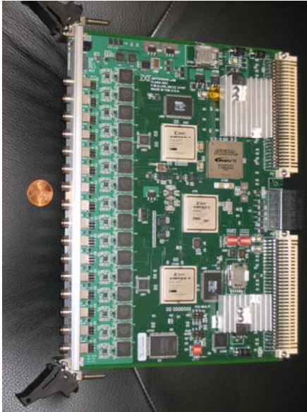
Figure 3: The 250 MSPS fADC
