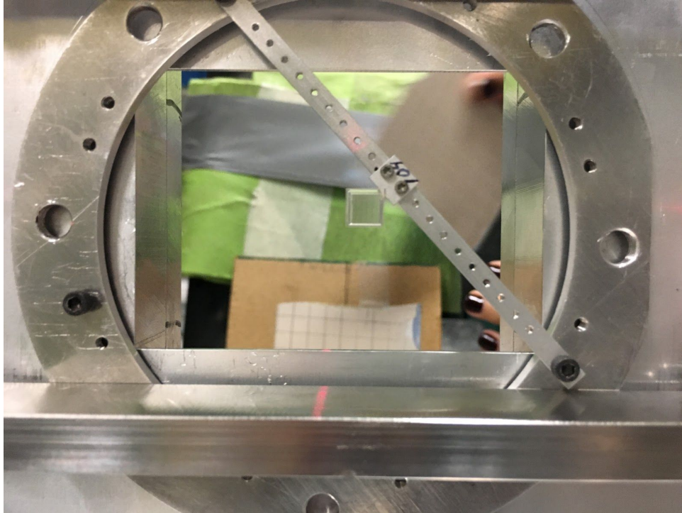
Photo of JD-104 mounted on target holder, for its Scan #1 configuration (12 o' clock, facing upstream).
